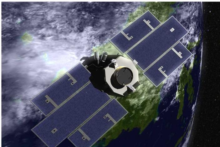
The main instrument on CloudSat is the Cloud Profiling Radar (CPR), a 94-GHz nadir-looking radar that measures the power backscattered by clouds as a function of distance from the radar.
