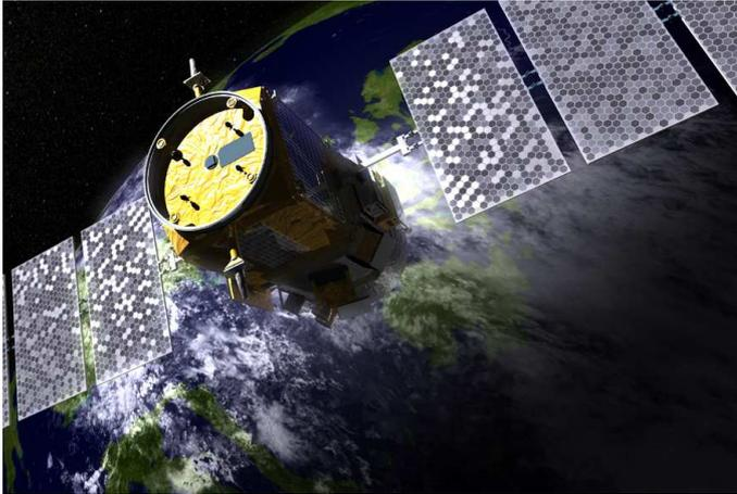
Passive and active remote sensing Instruments onboard the CALIPSO satellite will monitor aerosols and clouds 24 hours a day.
